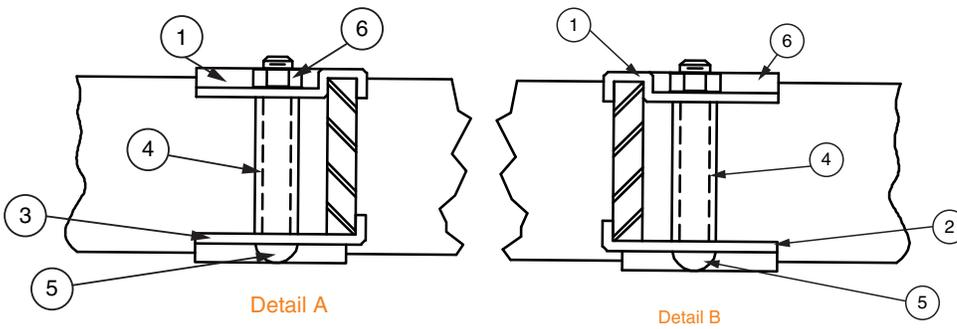
**ATTACHING VERTICAL CABLE RACK TO 1 SIDE BAR OF HORIZONTAL CABLE RACK**
