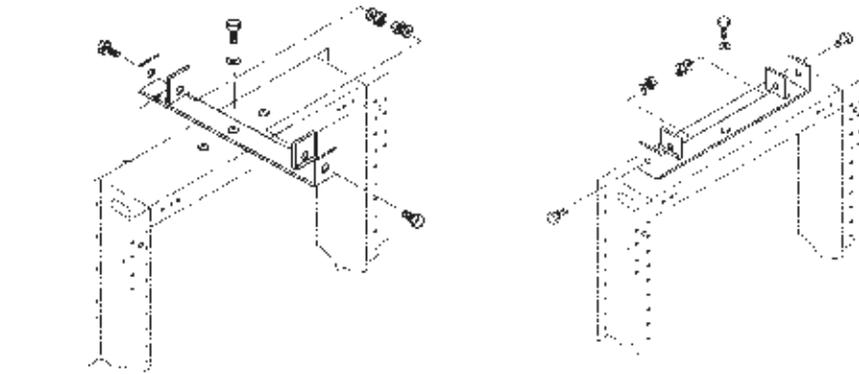
**FASTENING CABLE RACK TO FLOOR OR WALL**
