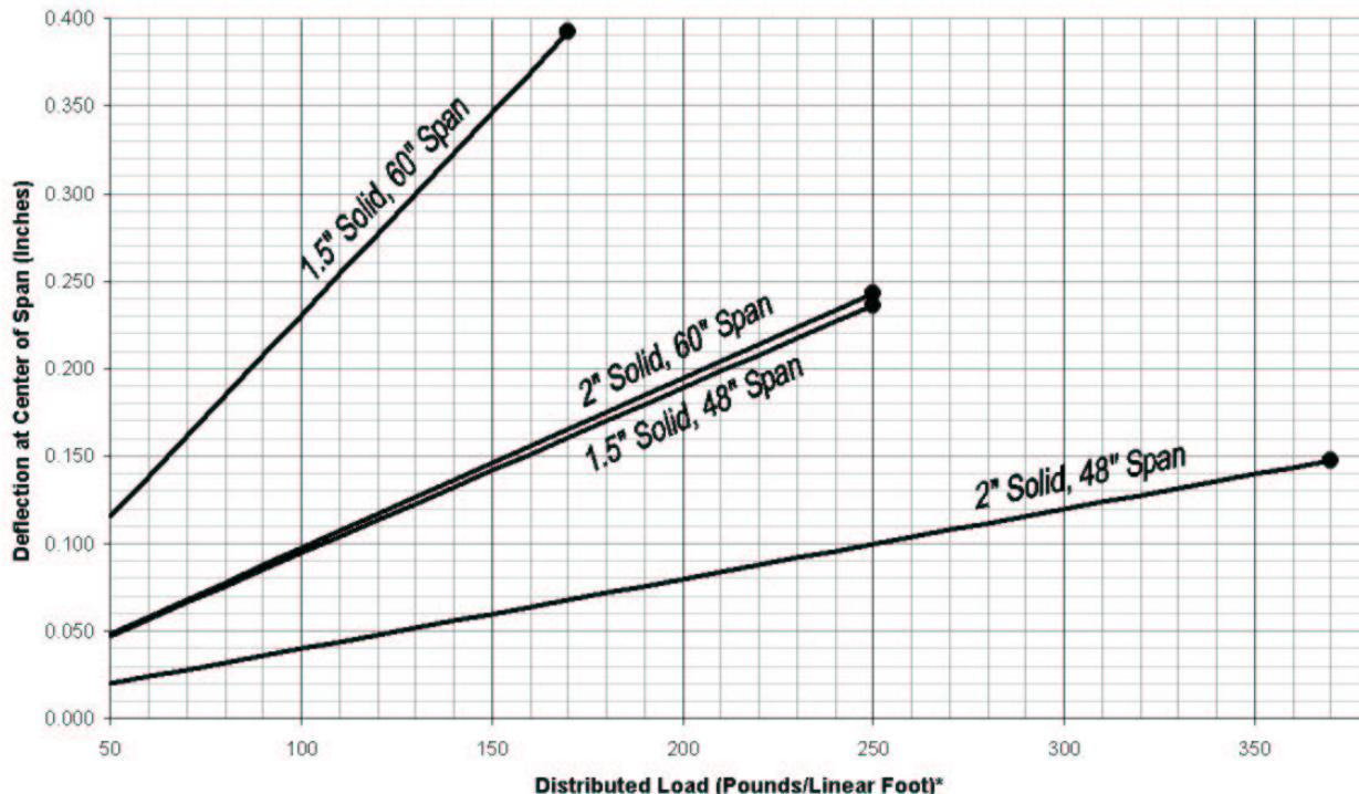
This chart shows the expected deflection of 12" or narrower channel type cable rack spanning 48 or 60 inches. This data has been calculated and verified by testing. The data labels are as follows:
