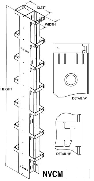
Newton Vertical Cable Management (NVCM) systems offer spacesaving, high quality, and lightweight cable management options. They are double-sided, mount between equipment racks (both Newton's and others'), and all edges are protected against possible cable wear and abrasion. Available in narrow (3.65") and wide (6.00") widths, and various heights (see ordering chart below).
