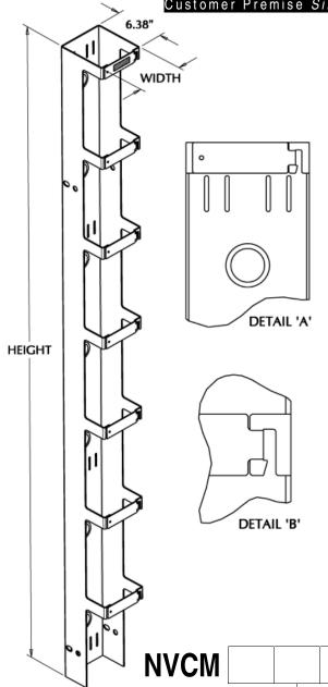
Newton Vertical Cable Management (NVCM) systems offer spacesaving, high quality, and lightweight cable management options. They are single-sided, mount between equipment racks (both Newton's and others'), and all edges are protected against possible cable wear and abrasion. Available in narrow (3.65") and wide (6.00") widths, and various heights (see ordering chart below).
