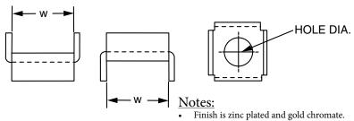
part number Hole Opening Bolt 0030320110 1-1/2" 13/32 3/8" hole 0030320210 1-1/2" 17/32 hole 1/2" Ordering Table 0030320310 1-1/2" 21/32 hole 5/8" 0030320410 1-7/8" 13/32 hole 3/8" 0030320510 1-7/8''17/32 hole 1/2" 5/8" 0030320610 1-7/8" 21/32 hole 2023960810 1-7/8″ 21/32 Slot 5/8"
