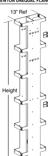
Newton Unequal flange Cabling Section (NUCS) systems offer space-saving, high quality, and lightweight cable management options. They are double-sided, mount between "unequal flange" and "netbay" equipment racks and all edges are protected against possible cable wear and abrasion. Available in narrow (3.65") And wide (6.00") Widths.
